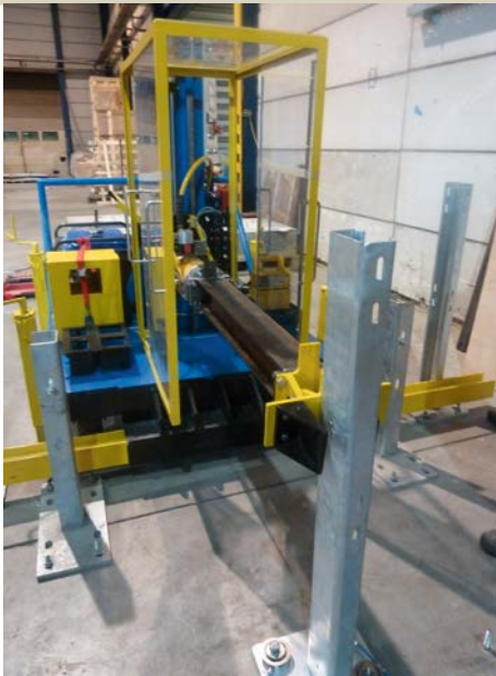
Equipment to test soils and anchor plates
