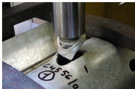
Test of bolted joints
