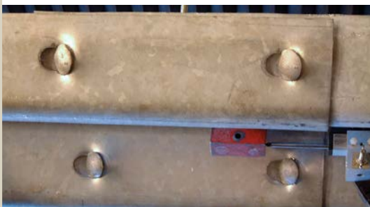
Beam-to-beam connection test
