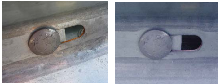
Safety barrier by Mieres Tubos/Grupo Condesa coated in Magnelis® ZM310 (steel thickness 3 mm). Exposure was started outdoors in September 2011 (left). Note the self-healing effect on the perforations in October 2013 (right).
